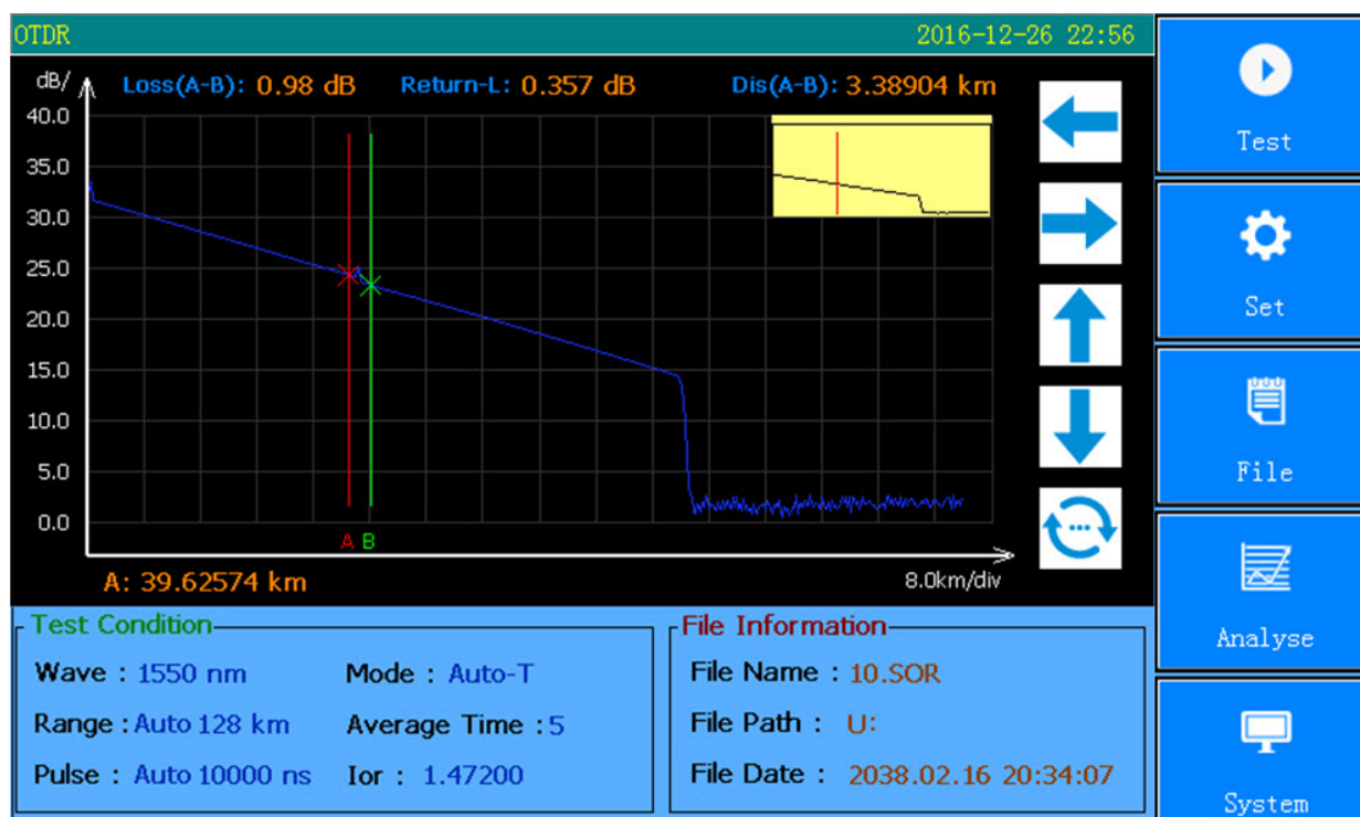
Fig.3-9 Connection Loss Measurement
